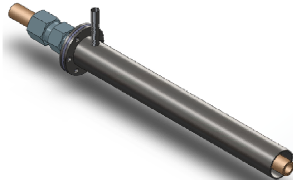
3 kWth Reactor (Endothermic + Exothermic) (2 in Dia X 14 in. long)
